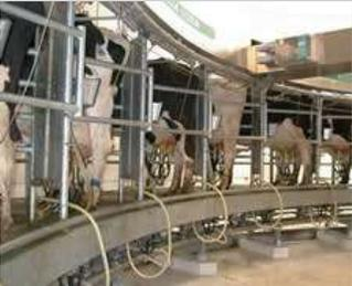
the milk causes a slug to form, drastically limiting the amount of vacuum that can get to the teat end of the cow. Lifting milk can be found in many different places in the milking
